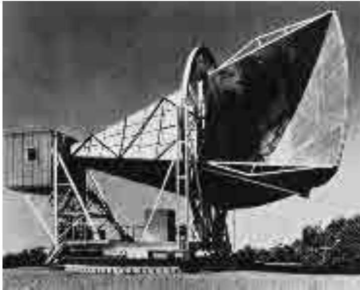
Radio waves thought to have originated in the primeval fireball that marked the start of the expansion of the universe were first detected by Arno Penzias and Robert Wilson with a sensitive receiver attached to this 15-m-long antenna at Holmdel, New Jersey.
